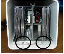
3. The plate rack is removed by lifting it up and pulling it out.
