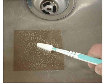
4. If the generator needs to be put back in service immediately you will need an oven or other source of heat to dry the mica and screens. If using an oven set the temperature at about 200° F and place the mica and screens on the middle rack for approximately 1-2 hours. If there is no rush or you do not have access to an oven, place the mica and screens in a very warm dry place such as on an operating base board heater to dry overnight.
