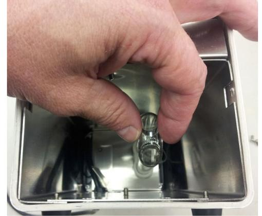
4. If you are replacing the tubes go to step #5 otherwise, take the tubes and use an alcohol moistened paper towel or a lightly soap and water moistened paper towel to wipe the tubes down and remove any deposits. If soap water is used then a second wiping with a clean water moistened paper towel will be required to remove the soap.
