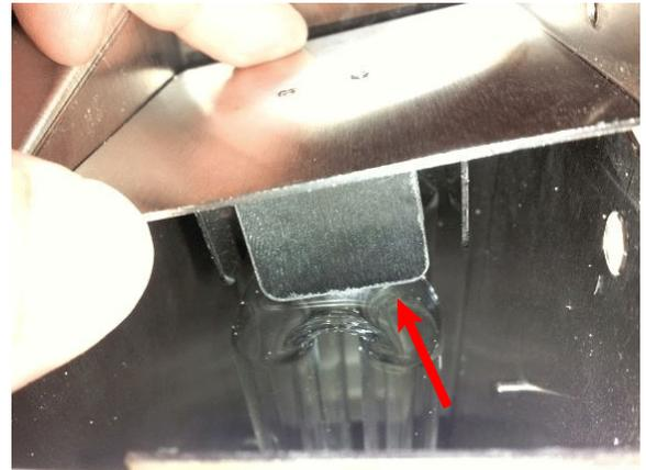
10. Replace the end cap and re install the 2 end cap screws. The unit is now ready for use.
