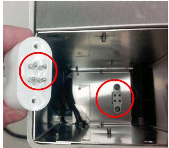
9. When reinstalling the light deflector ensure that the tube is inserted into the tube holder bracket that is part of the light deflector.
