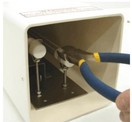
4. To remove the tube lift the end up out of the stainless support and pull while wiggling the tube back and forth being careful not to break it on the steel supports.
