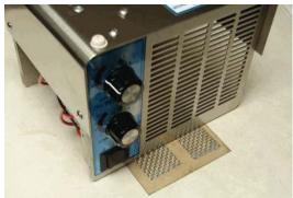
4. If the generator needs to be put back in service immediately you will need an oven or other source of heat to dry the mica and screens. If using an oven set the temperature at about 150° F (lowest setting) and place the mica and screens on the middle rack for approximately 1-2 hours.
