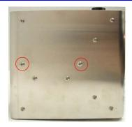
3. With the 2 screws removed the stainless plate that holds the mica will come out of the generator.
