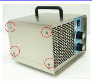
2. While holding the stainless steel plate, as shown in the first picture to the right, remove the 2 Philips screws indicated in the second picture.
