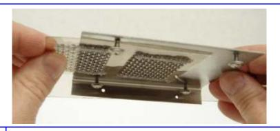
7. Once the mica/screen is in place tighten the 4 screws to hold the mica in place on the stainless plate.
