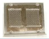
8. Use an alcohol soaked paper towel or something similar to wipe down any other areas of the machine that are dirty such as inside the ozone generator chamber. Clean the filters with dish soap and rinse thoroughly with water and allow to dry.
