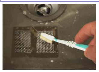
3. NOTE: Try to be very careful not to remove the screen from the mica. If the screen comes off the mica sheet this can be repaired by first cleaning the mica with alcohol and then putting a very thin amount of silicone on the existing silicone that is stuck to the screen then re place them on the mica in the same position as it was originally.
