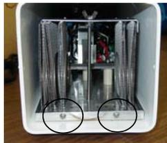
11. To access the filter remove the end cap at the air input end of the ozone generator in the same way the output cap was removed in step one. The filter may be washed with soapy water or replaced with a new filter available thru your CAMI supplier. If another brand of filter is used please ensure that it has good air flow or else the ozone generator could overheat due to lack of cooling.
