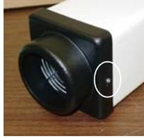
2. The generator plate rack is secured by two screws that are located inside the unit behind the end cap instead of on the bottom as indicated in the original manual.
