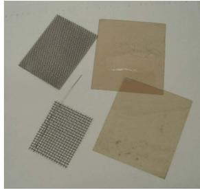
3. Take mica and stainless screens and clean in the sink using dish soap and an old toothbrush. If the plates have not been cleaned for a long time, it is important to use the tooth brush to help remove the flaking mica. Rinse with clean clear water.
