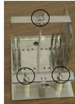
5. Once the bar and contact bracket are removed, remove the plates by lifting them straight up as shown.
