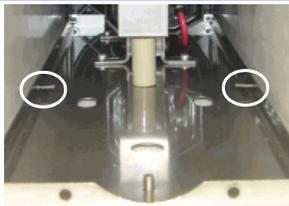
10. Replace the plate rack, reinstall the screws that hold the rack in place and reinstall the end cap and screws.
