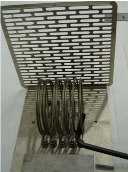
7. Slip the plate in between the springs, make sure that the spring does not go up in the middle of the plate as shown.
