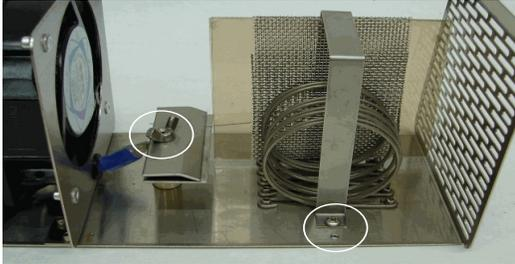
4. Once the plate hold down bracket and HV contact bar are removed, remove the plates by lifting them straight up as shown.
