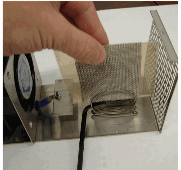
8. Re install the HV clamp and plate hold down bracket that was removed in step 2.
