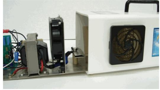
3. Remove the two Philips screws from the plate hold down bracket and the wing nut from the HV clamp as indicated.
