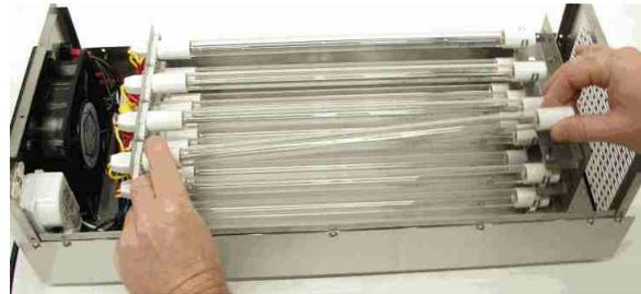
6. To remove the second and third row of tubes you will need to first remove the tube support bracket after removing the tubes. This bracket is removed by removing 2 screws from each as indicated in the image. Then repeat the removal of the hold down brackets, ties, and tubes as in step 4, 5, & 6 for 2<sup>nd</sup> and 3<sup>rd</sup> rows.
