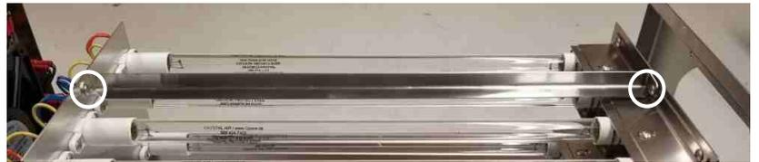
4. Remove the 2 screws indicated in the image. Remove the tube hold down bracket.
