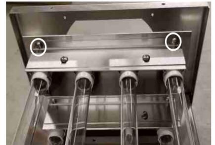
5. To remove the tube lift the end and pull while wiggling the tube back and forth being careful not to break it on the steel support / light guard.
