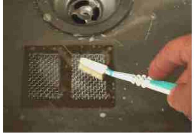
3. **NOTE:** Try to be very careful not to remove the screen from the mica. If the screen comes off the mica sheet this can be repaired by first cleaning the mica with alcohol and then putting a very thin amount of silicone on the existing silicone that is stuck to the screen then re place them on the mica in the same position as it was originally.
