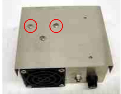
3. With the 2 screws removed the stainless plate that holds the mica will come out of the generator.
